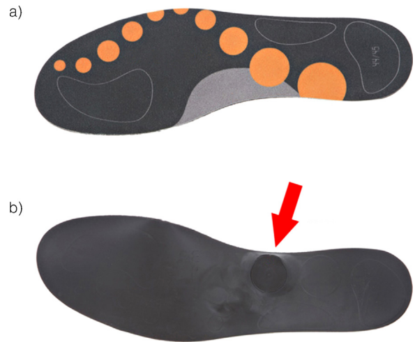
Fig. 1. Standard right OpenGo insole (Moticon GmbH, Munich). Artificial leather cover. 13 capacitive pressure sensors, accelerometer and thermometer. (a) View from below. (b) View from above. The round opening for a regular 3,7V Li-ion battery can be seen (red arrow). (For interpretation of the references to colour in this figure legend, the reader is referred to the web version of this article.)
