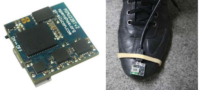
Figure 8: IMU attached to the tip of the foot.
